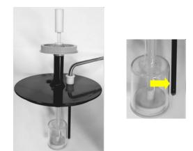
The heat generated from the reaction is absorbed by the calorimeter (container + stirrer + water (solutions) + temperature detectors), raising its temperature by  $\Delta T$ ;
